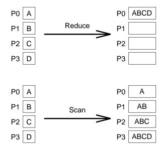
Schematic representation of collective data movement in MPI
