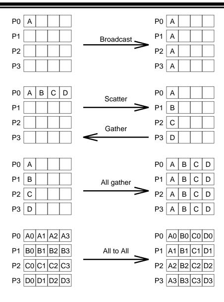
Schematic representation of collective data movement in MPI
