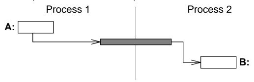
But this requires that either that MPI\_Send not return until the data has been delivered *or* that we allow a send operation to return before completing the transfer. In this case, we need to test for completion later.
