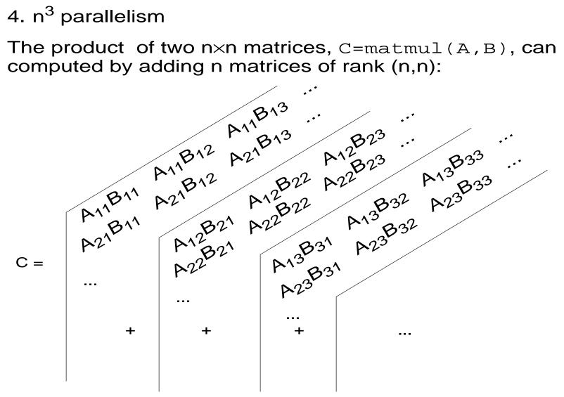
These n matrices of rank (n,n) can be computed by multiplying (element-by-element) two three-dimensional arrays of rank(n,n,n).
