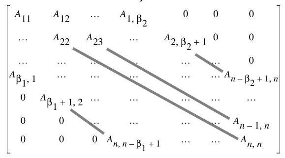
For a small band, for example,  $\beta_1 = \beta_2 = 3$ , the algorithm discussed before for matrix-vector multiplication is not efficient.
