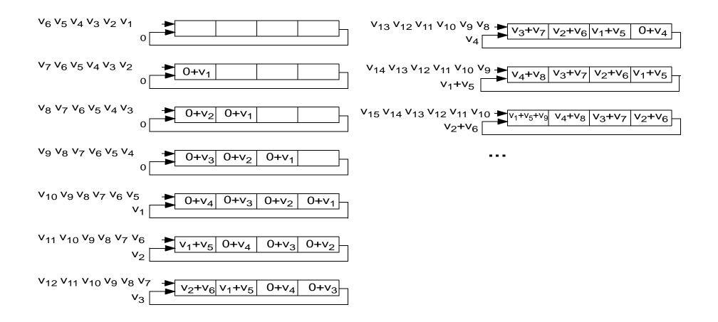
At the end of the process, there will be  $s_{\#}$  (the number of stages used by the pipe to perform the # operation) partial results which should be added to get the final result. The time to get the final result is therefore:
