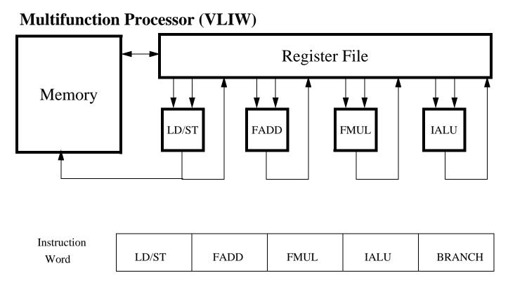
• Array processors. Multiple arithmetic units
