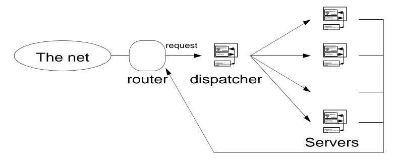
Another example is the workstation cluster at Fermilab, which consists of about 400 Silicon Graphics and IBM workstations. The system is used to analyze accelerator events. Analyzing any one of those events has nothing to do with analyzing any of the others. Each machine runs a sequential program that analyzes one event at a time. By using several machines it is possible to analyze many events simultaneously.
