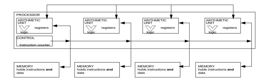
Illiac IV is the earliest example of this type of machine. Each arithmetic unit (processing unit) of the Illiac IV was connected to four others to form a two-dimensional array (torus).
