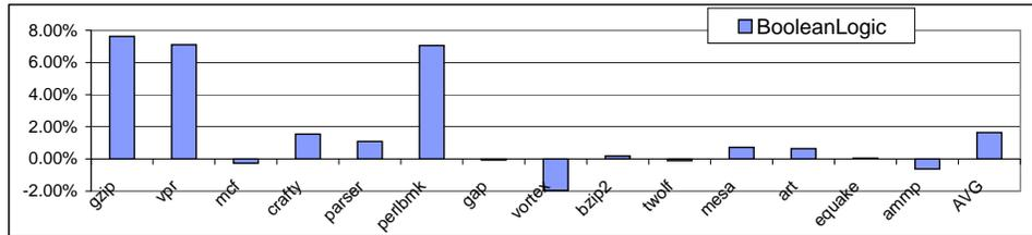
Fig. 8. Performance speedup with boolean logic optimization compared to baseline replication
